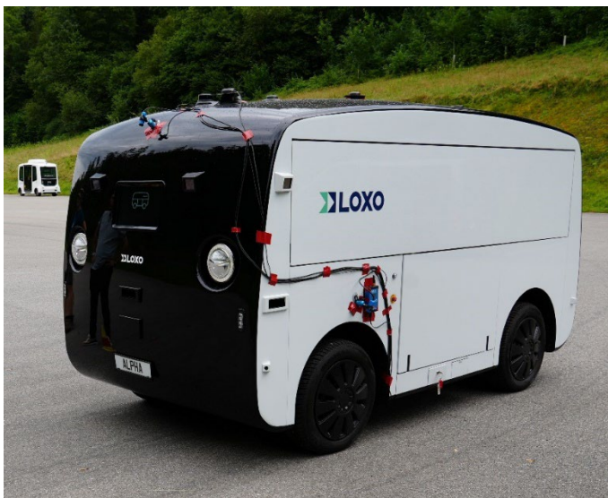
Figure 78: Antenna and camera positioning on LOXO Alpha
