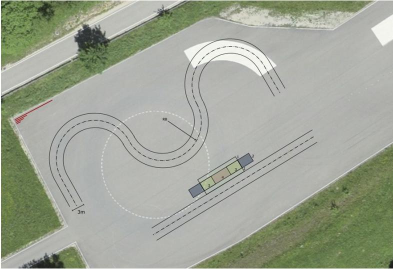
Figure 68: Aerial view, DTC test drive area, slalom and parking testing tracks
