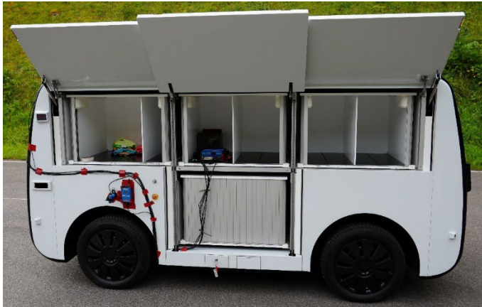
Figure 77: Measurement equipment on LOXO Alpha
